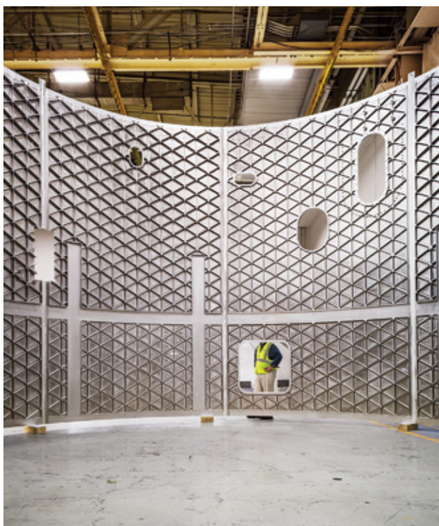
BARREL SEGMENTS stacked and welded together to form a tall cylinder will serve as the shell of the SLS's core stage. Inside that shell, a tank each of liquid hydrogen and liquid oxygen will carry the rocket's fuel. At NASA's Michoud Assembly Facility, engineers are now producing "confidence" barrels to test the strength of the components.
