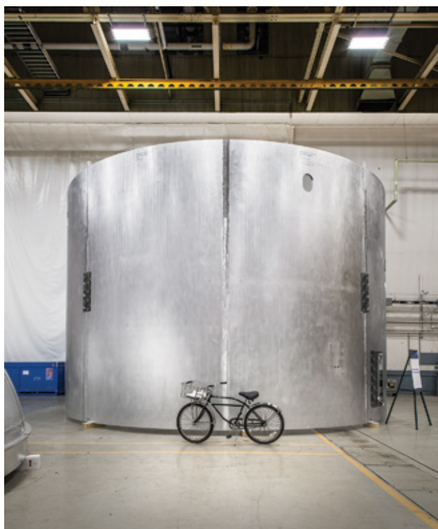
BARREL SEGMENTS stacked and welded together to form a tall cylinder will serve as the shell of the SLS's core stage. Inside that shell, a tank each of liquid hydrogen and liquid oxygen will carry the rocket's fuel. At NASA's Michoud Assembly Facility, engineers are now producing "confidence" barrels to test the strength of the components.
